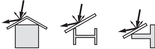
Fig. 16: Cover flat, large-area profiles with deflectors
