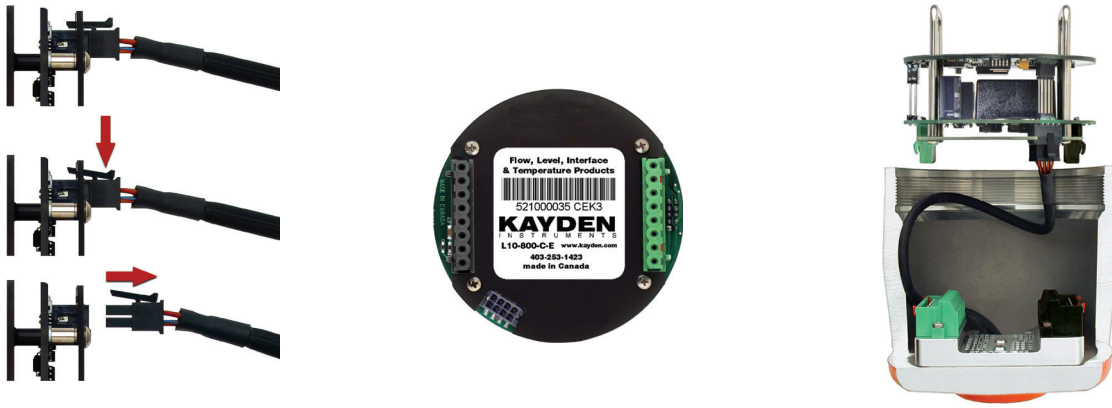
Figure 10 - Disconnecting Sensor Connector from the Electronics Module
