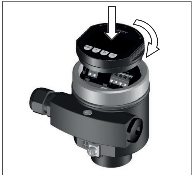
Fig. 11: Installing the display and adjustment module in the electronics compartment of the single chamber housing
