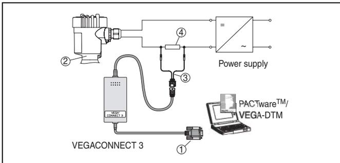
Fig. 13: Connecting the PC to the signal cable
