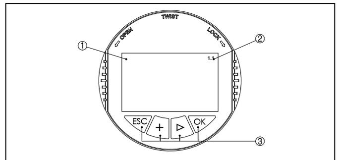
Fig. 11: Indicating and adjustment elements
