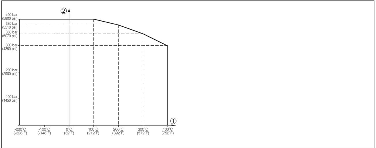
Fig. 16: High temperature version: Process pressure - product temperature
