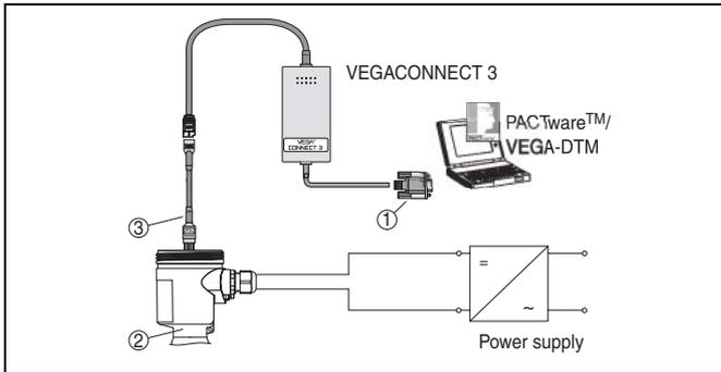
Fig. 12: PC connected directly to the sensor
