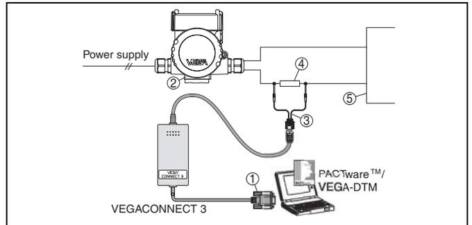
Fig. 14: Connecting the PC to the signal cable
