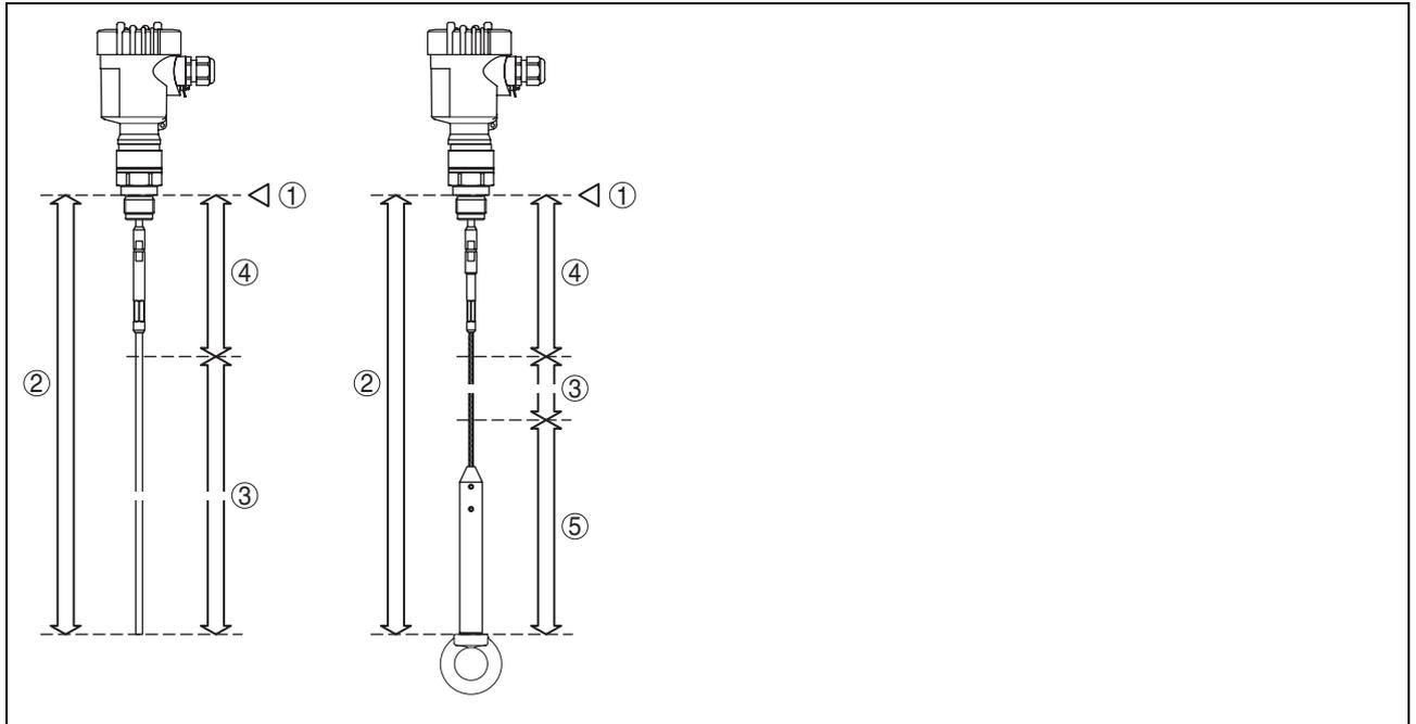
Fig. 15: Measuring ranges of VEGAFLEX - cable and rod version e.g. VEGAFLEX 61
