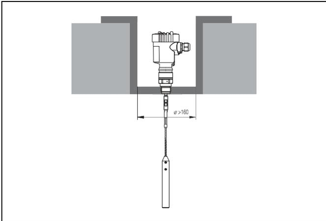
Fig. 7: Installation in concrete silos
