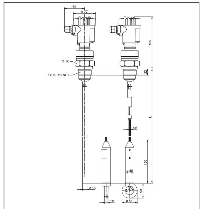
Fig. 23: VEGAFLEX 62 - cable and rod version with thread
