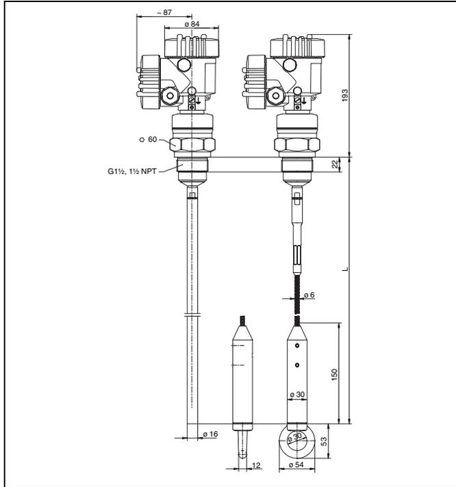
Fig. 24: VEGAFLEX 62 - cable and rod version with thread (double chamber housing)
