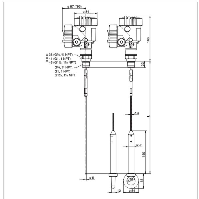
Fig. 22: VEGAFLEX 61 - cable and rod version with thread (double chamber housing)
