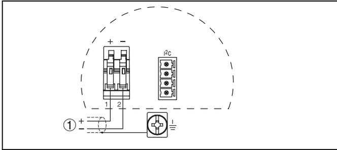
Fig. 9: Connection HART two-wire, Profibus PA, Foundation Fieldbus
