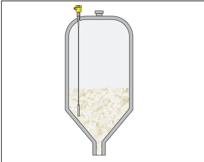
Fig. 2: Level measurement of plastic granules with VEGAFLEX 61
