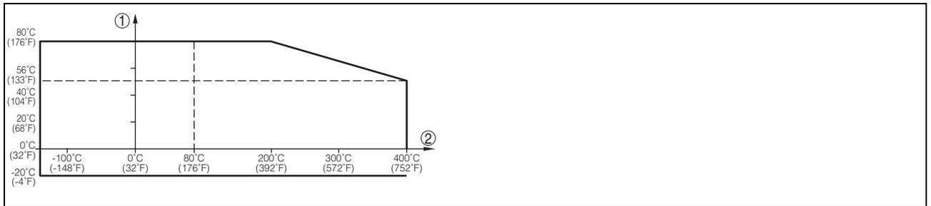
Fig. 18: Ambient temperature - product temperature (version -200 ... +400 °C/-328 ... +752 °F)
