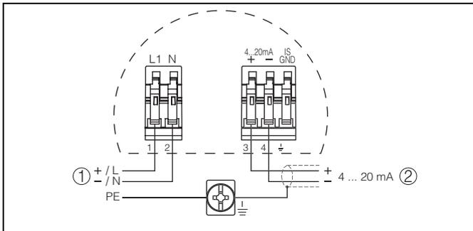
Fig. 10: Connection 4 ... 20 mA/HART four-wire
