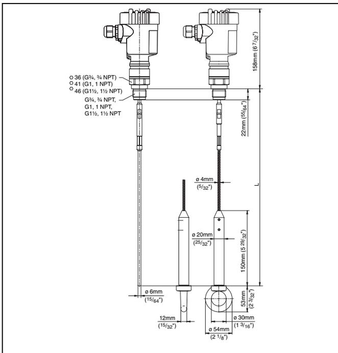
Fig. 21: VEGAFLEX 61 - cable and rod version with thread
