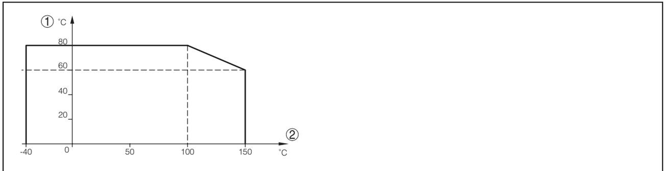
Fig. 17: VEGAFLEX - Ambient temperature - Product temperature
