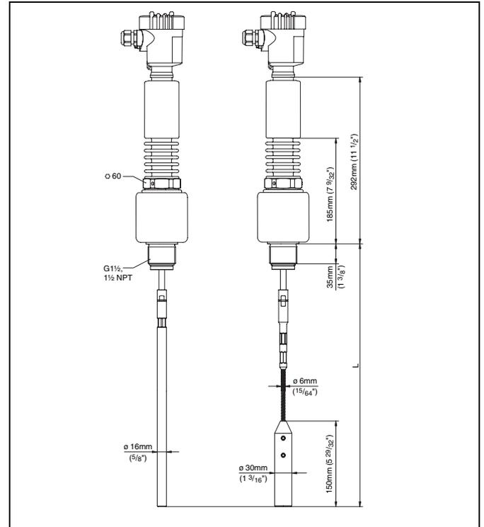
Fig. 25: VEGAFLEX 66 - rod, cable version -200 ... +400 °C (-328 ... +752 °F)
