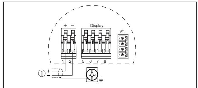
Fig. 8: Connection HART two-wire, Profibus PA, Foundation Fieldbus
