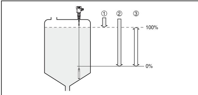
Fig. 4: Measuring range (operating range) and max. measuring distance
