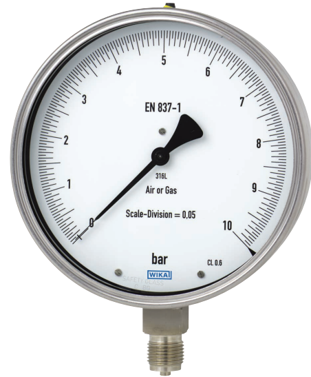
Test gauge, stainless steel, model 332.50
