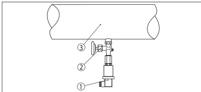
Fig. 5: Measurement setup for the process pressure measurement of liquids in pipelines
