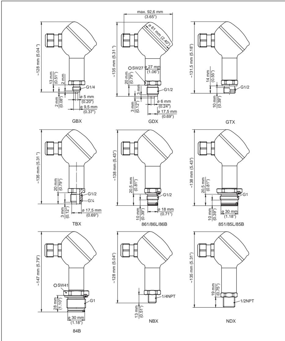
Fig. 20: VEGABAR 17 terminal housing, GBX = G $\frac{1}{4}$  B manometer connection, GDX = G $\frac{1}{2}$  B manometer connection, GTX = G $\frac{1}{2}$  A according to DIN 3852-E, TBX = G $\frac{1}{2}$  B, inside G $\frac{1}{4}$  B, 84B = G1 B front-flush max. 25 bar, 851/85L/85B = G1 B front-flush with O-ring up to 1.6 bar, 861/86L/86B = G $\frac{1}{2}$  B front-flush with O-ring > 1.6 bar, NBX =  $\frac{1}{4}$  NPT thread, NDX =  $\frac{1}{2}$  NPT thread
