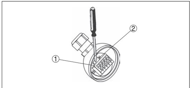
Fig. 14: Adjustment of zero and span
