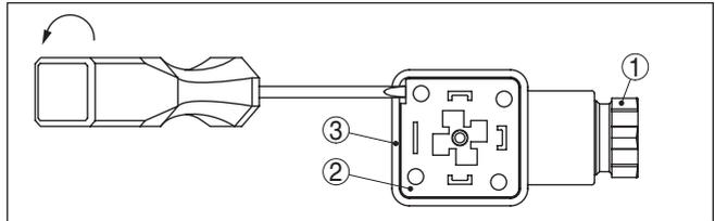
Fig. 6: Loosen the plug insert
