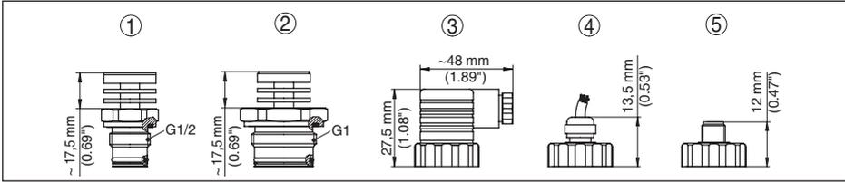
Fig. 21: VEGABAR 17 - cooling elements, plug, cable outlet
