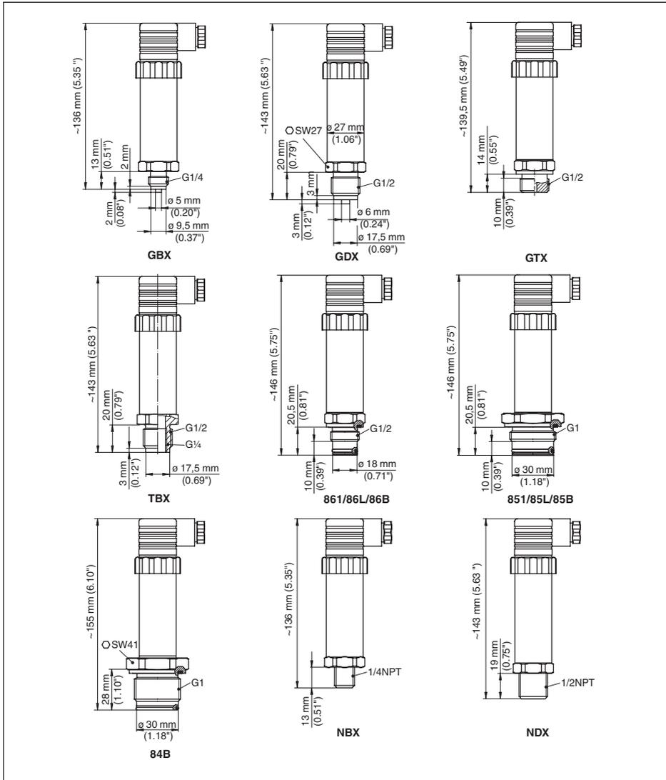
Fig. 19: VEGABAR 17 standard housing, GBX = G $\frac{1}{4}$  B manometer connection, GDX = G $\frac{1}{2}$  B manometer connection, GTX = G $\frac{1}{2}$  A according to DIN 3852-E, TBX = G $\frac{1}{2}$  B, inside G $\frac{1}{4}$  B, 84B = G1 B front-flush max. 25 bar, 851/85L/85B = G1 B front-flush with O-ring up to 1.6 bar, 861/86L/86B = G $\frac{1}{2}$  B front-flush with O-ring > 1.6 bar, NBX =  $\frac{1}{4}$  NPT thread, NDX =  $\frac{1}{2}$  NPT thread
