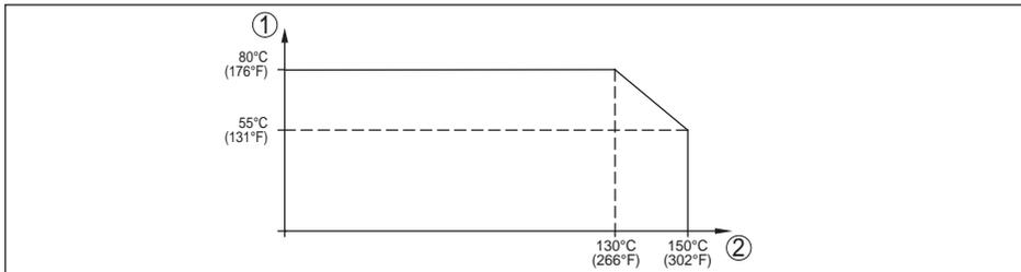
Fig. 17: Temperature derating VEGABAR 17
