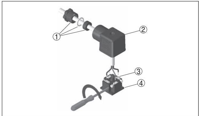
Fig. 7: Connection to the screw terminals
