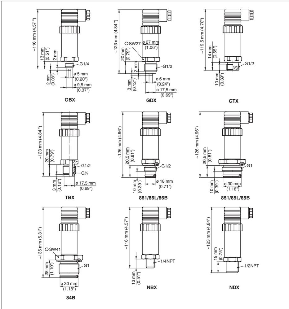
Fig. 18: VEGABAR 17 standard housing, GBX = G $\frac{1}{4}$  B manometer connection, GDX = G $\frac{1}{2}$  B manometer connection, GTX = G $\frac{1}{2}$  A according to DIN 3852-E, TBX = G $\frac{1}{2}$  B, inside G $\frac{1}{4}$  B, 84B = G1 B front-flush max. 25 bar, 851/85L/85B = G1 B front-flush with O-ring up to 1.6 bar, 861/86L/86B = G $\frac{1}{2}$  B front-flush with O-ring > 1.6 bar, NBX =  $\frac{1}{4}$  NPT thread, NDX =  $\frac{1}{2}$  NPT thread
