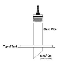
diameter pipe and shortest length possible. As a general rule, the diameter of the pipe should be 1/2 the length. The pipe ID must remain the same through it's entire length.
