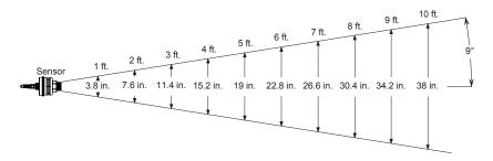
Typical beam spread of an ultrasonic sensor operating at maximum sensitivity setting.
