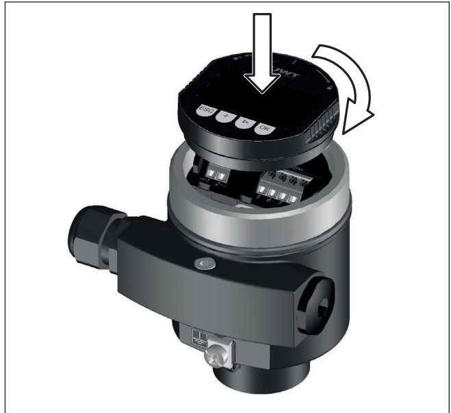
Fig. 13: Installing the display and adjustment module in the electronics compartment of the single chamber housing
